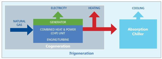
Figure 3. Principles of Natural Gas Trigeneration
