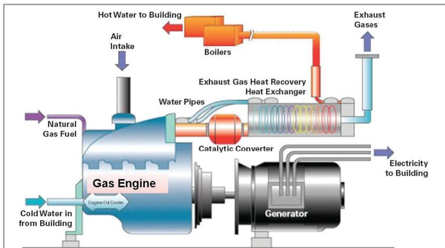
Figure 1. Inside a Combined Heat and Power Unit
