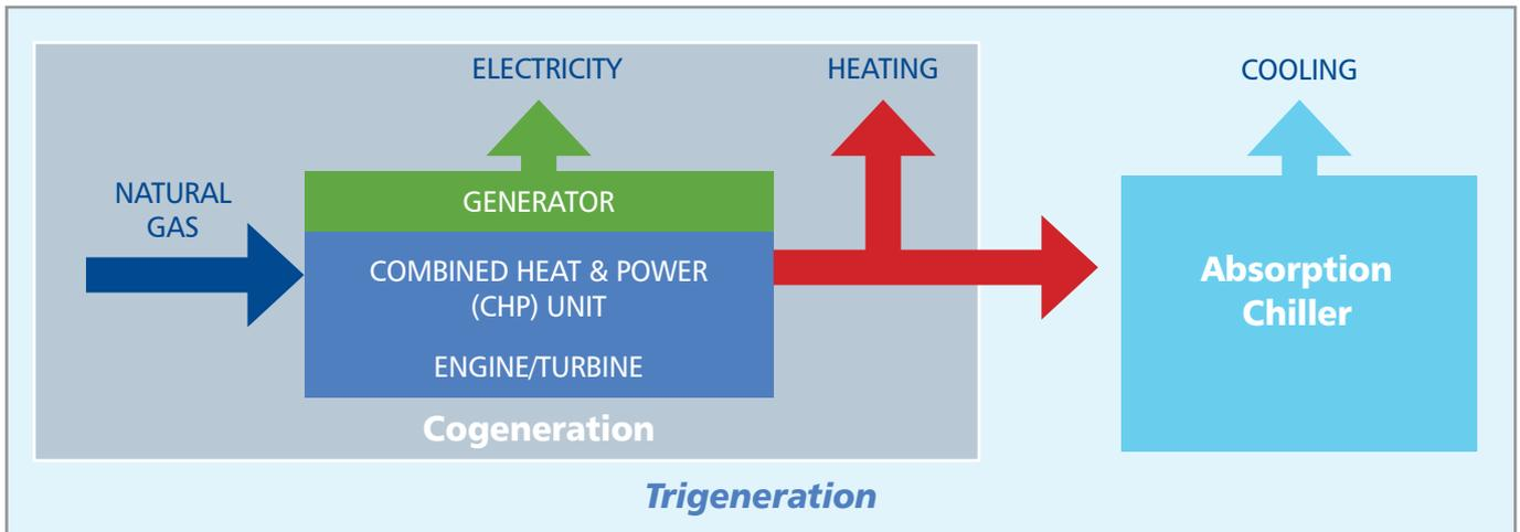
Figure 3. Principles of Natural Gas Trigeneration
